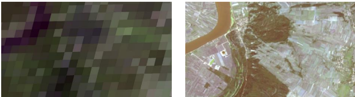
Figure 6: Comparison of low spatial resolution MODIS data (left) and high spatial resolution Sentinel-2 data (right)
